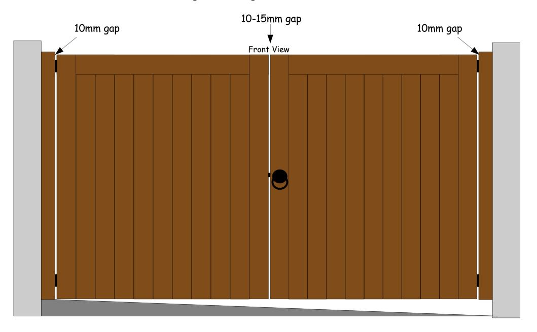
• Finally screw your hinges onto the wall posts, adjust the hinges to get the gate level and fit the closing catch.
