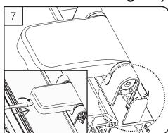
To release cover remove security screw from under the hinge and then insert 5mm blade screwdriver and twist. Use small blade screw driver to release cover caps.
