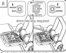
To adjust lateral position, first turn the unlock screw a 1/4 turn. Then use the adjustment screw to adjust up to 5mm in either direction. Finally tighten lock screw.
