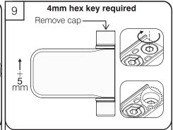
Height adjustment: Using a 4mm hex key turn the screw down to lift the hinge by up to 5mm.
