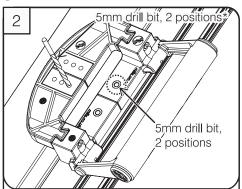
Using the Mila jig for alignment, drill holes for frame part and if fitting \*optional fixing pegs drill the sash part choosing the most suitable position for the pins on the profile.
