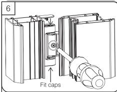
Open the sash to gain access to the security screw location and using screw provided fix in place to secure cover and hinge pin.
