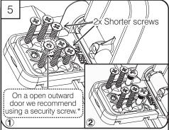
(1) Secure using 4x long screws & 2x short screws. Or (2) Use 4x long screws & 2x supplied fixing pegs. Close cover.
