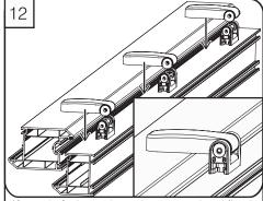
Alternatively the sash can be removed and fitted in the closed position by removing the security screws and hinges pins and then lifting the sash
