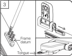
Fit the frame datum into the drilled 5mm holes and screw in place. Take hinge and align the aperture in the frame part and slide into position. ift sash cover and remove tongue.
